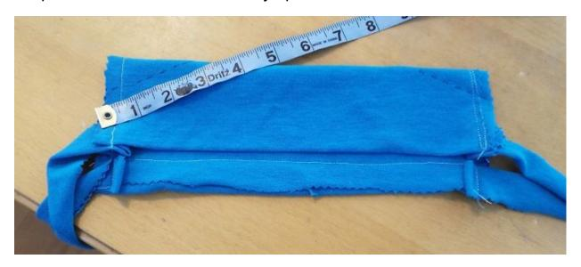
The position of the gussets are pictured above. The hem with the copper strip is at the top side.
